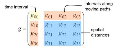
If I have space-time coordinates of two events, I can use this to tell distances and times. This little part gives the time interval, this little block tells me how to calculate spatial differences for things that are rest, and these other two little blocks tell me how to calculate intervals along moving paths. Now it is the nature of the way we define a coordinate system that I can always find one system that's moving at the correct speed to make the metric end up looking like this.
